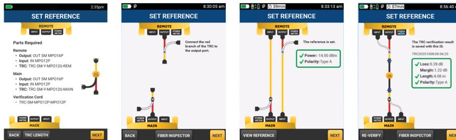
The Set Reference Wizard simplifies the setup process and greatly reduces errors. Left: List of all accessories required for the selected test are displayed. Middle left: The Wizard displays the steps and verifies that each has been performed. Middle right: The CertiFiber Max OLTS provides a 1-jumper reference setting for all MPO 12/16/24 and MMC 16/24 pinned and unpinned cables. Right: Reference values are checked for compliance and stored as proof of proper setting.
