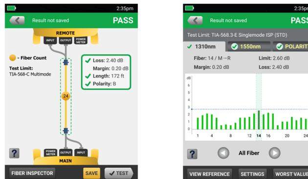
Left: Results screen indicates PASS or FAIL results and shows worst margin, length, polarity, number of fibers tested, and test limits. Touching the fiber under test (marked “24” in this case) brings up the detailed results by fiber (right) and wavelength along with polarity detail.
