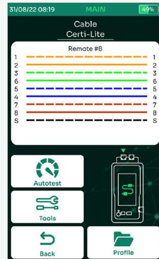
Figure 5 - Wiremap with Remote ID#8 Identified
