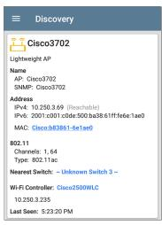
The linked and underlined Cisco MAC address in the screen image above opens the Wi-Fi app's AP Details screen, where you can view the other wireless attributes associated with the Lightweight AP. The Nearest Switch and Wi-Fi Controller links open a Discovery app Details screen for those devices.
