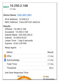
**Device Name**: The discovered name of the DHCP Server, or, if no name could be discovered, the IP address
