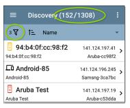
Back on the main Discovery screen, the screen title shows the number of filtered devices out of the total discovered devices (in the image above, 152 filtered devices out of 1308 total).
