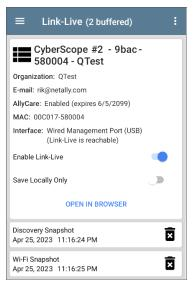
The buffered files displayed automatically upload to Link-Live.com once your CyberScope connects to an active network
