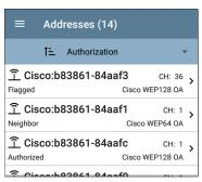
To reset a device's User Name and/or Authorization to the unassigned defaults, open the Name and Authorization dialog, clear the User Name field and leave it blank, and select the Unspecified Authorization. Then, tap OK.
