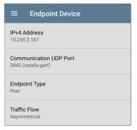
**IPv4 Address**: Tap the field to enter the IPv4 address of your endpoint device.
