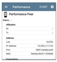
The Wired Test Port must be linked (by running an AutoTest Wired Profile) for the Performance Peer function to run. If the port is not linked, a Status message displays, "The wired test port is not linked."
