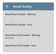
**Result Must Contain:** Specifies a value that the result must contain. Tap the field to open a text editor to enter a string or regex value. For example, the Graded Ports sample test uses this value:
