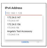
A drop-down list in the IPv4 Address dialog shows all the Test Accessories the CyberScope has discovered through the discovery process, as well as any Test Accessories that are claimed to the same Link-Live organization as your CyberScope.
