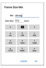
On the Frame Size Mix keyboard shown above, each letter (a through h) is associated with a frame size. The default pattern is "abceg," meaning the traffic pattern follow a repeating sequence of 64, 128, 256, 1024, and 1518 bytes.
