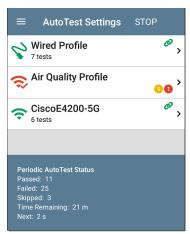
The Periodic AutoTest Status is summarized at the bottom of the AutoTest screens. Passes and failures are reported for each run of the entire Profile Group, rather than individual Profiles. Periodic AutoTests are skipped if the previous interval's test is still running when the next time interval occurs, such that the next run could not start.
