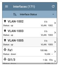
Like other Discovery list screens, the Interfaces list provides a number of Sort options, and the selected sort option affects the type of information displayed. The image above shows Interfaces sorted by Status (up or down). The image below shows Interfaces sorted by MAC Address, so each Interface's MAC address is displayed.
