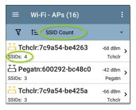
The selected Sort option displays in the Sort bar above the list, and the sort characteristic for each item is shown under the type icon and name. In the image above, the discovered APs are sorted by SSID Count, which is shown below each AP icon
