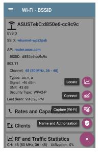
Tap Locate. This opens the Locate screen and causes your CyberScope to "listen" for the BSSID or Client wireless devices you want to find using either the internal antennas or the optional external antenna (sold separately or in kits).
