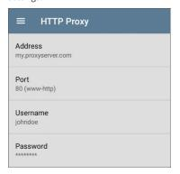
Tap each field to open a pop-up keyboard and enter the appropriate **Address** (you can enter a proxy name or an IPv4 address), **Port** (set to match the proxy port), **Username**, and **Password**. Tap **OK** to save your entries.
