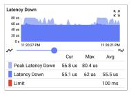
Latency (Up/Down): Latency is the amount of time it takes for a packet to go from the source to the endpoint or from the endpoint to the source (in milliseconds). Latency is calculated by averaging the thousands of latencies measured during each interval. One-way latency measurements consist of the round-trip measurements divided by two.
