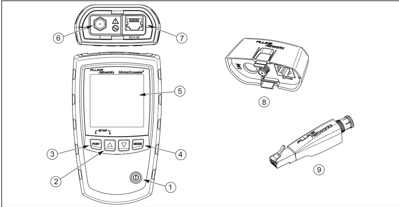
Figure 2. MicroScanner<sup>2</sup> Features
