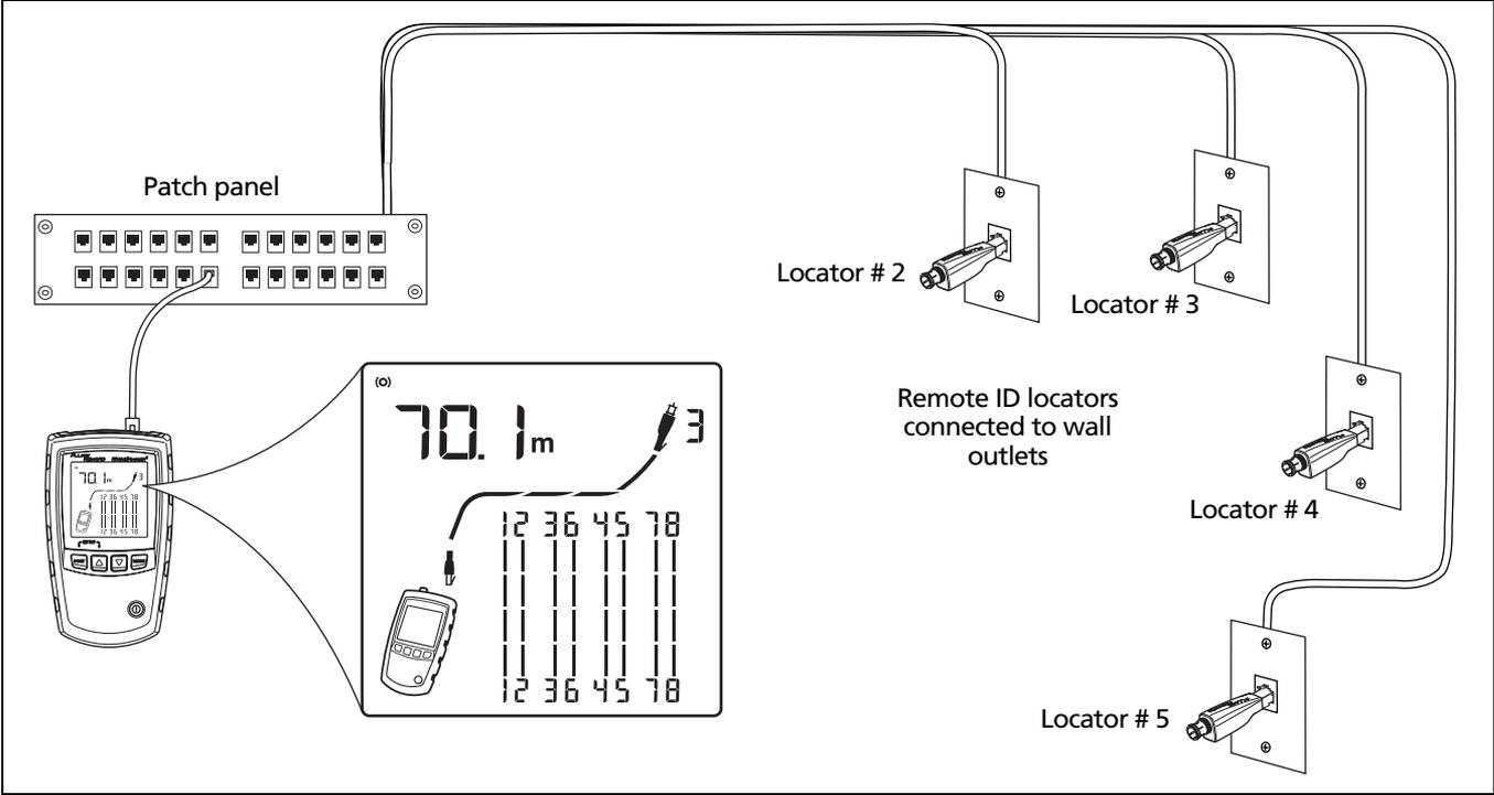
Figure 15. Using Multiple Remote ID Locators
