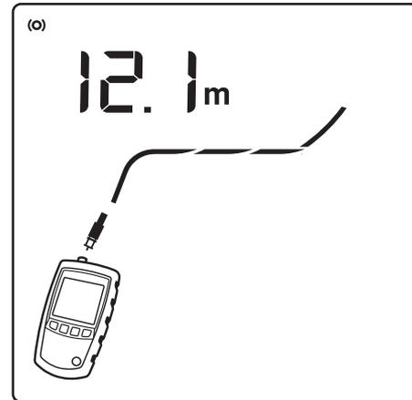
Figure 20. Open on Coaxial Cabling
