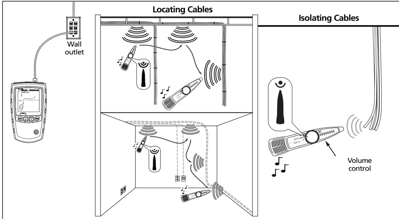
Figure 25. Using the Toner in IntelliTone Mode
