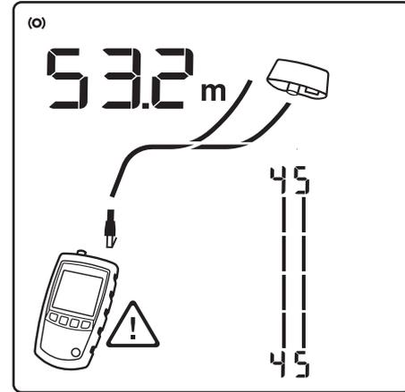
Figure 12. Bridge Tap Detected
